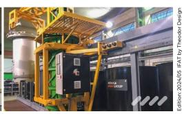
The actual process of slow thermal decomposition (PTR) takes about 2-3 hours and is proceeded in a closed system without air access = Non-oxidative thermal process. The PTR process itself is thermally stable and during the operation it continuously generates from the input charge three output fractions: gaseous, liquid and solid. Depending on the end use of these fractions, the PTR process outputs are certified as products.
